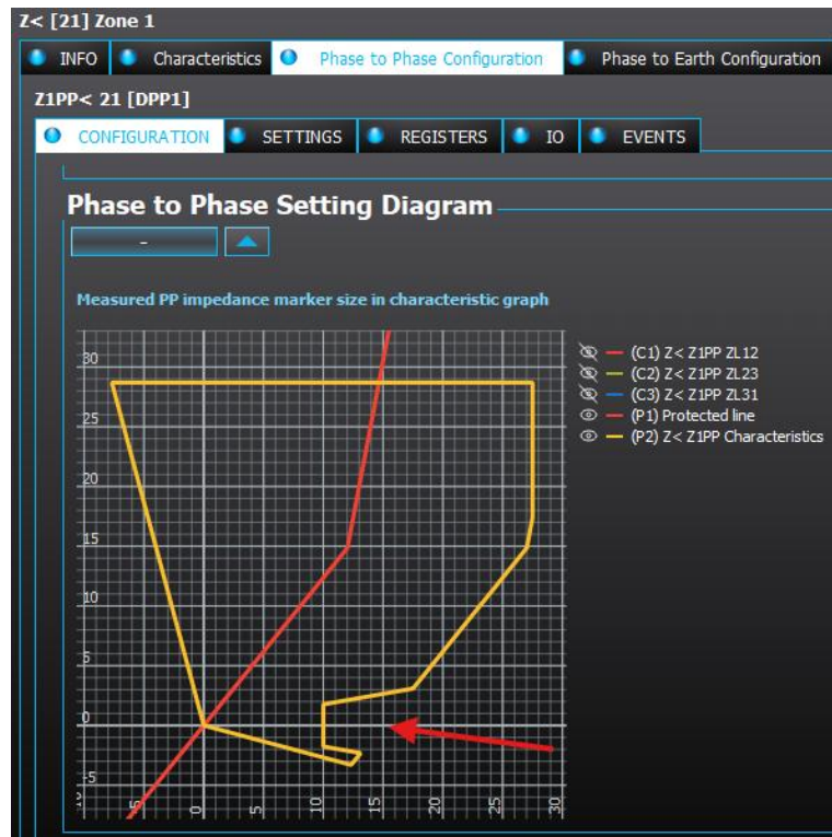
Figure 30. Load encroachment in zone characteristic.
