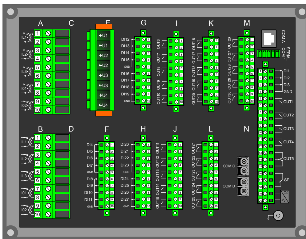
Figure. 7.1 - 204. Modular construction of AQ-X257-XXXXXXX-BBBCCCCCJ
