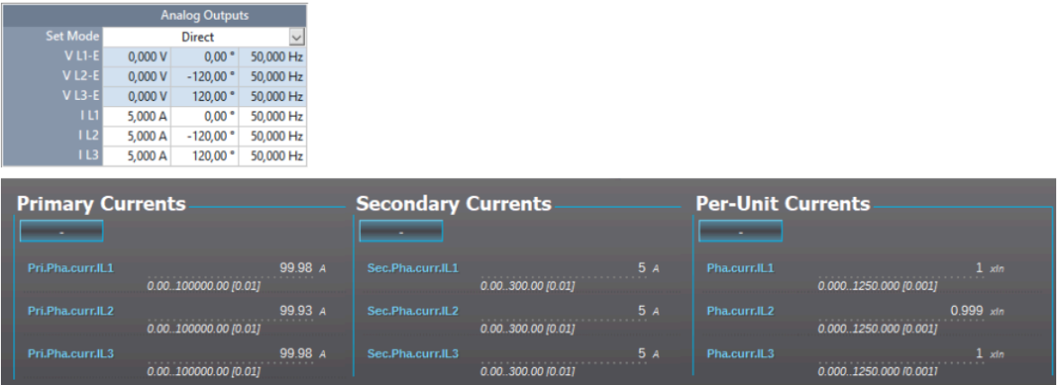
Figure. 4.2.1 - 8. Scalings display (based on the CT nominal).
