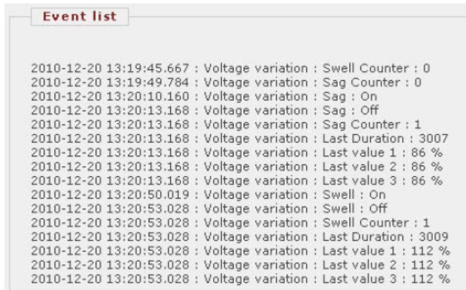
Figure. 9.10 - 144. Example sag and swell.
