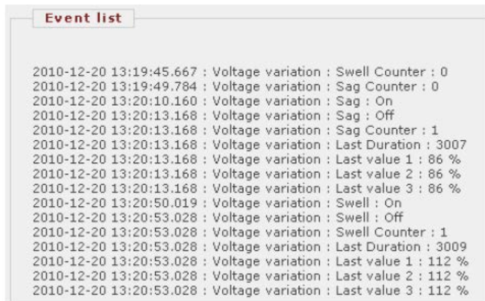
Figure. 9.10 - 132. Example sag and swell.
