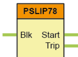
Figure. 8.18 - 97. The function block of the pole slip function.
