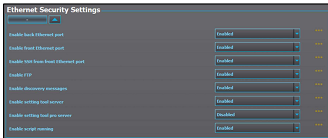
Figure 5. Ethernet security settings in AQtivate 200.
