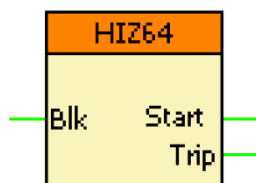
Figure. 6.3.14 - 88. The function block of the harmonic undervoltage protection function with offset characteristic.
