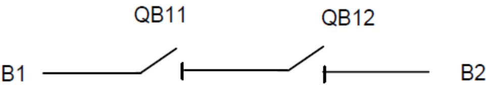
Figure. 8.4.2 - 62. Example sectionalizer topology.
