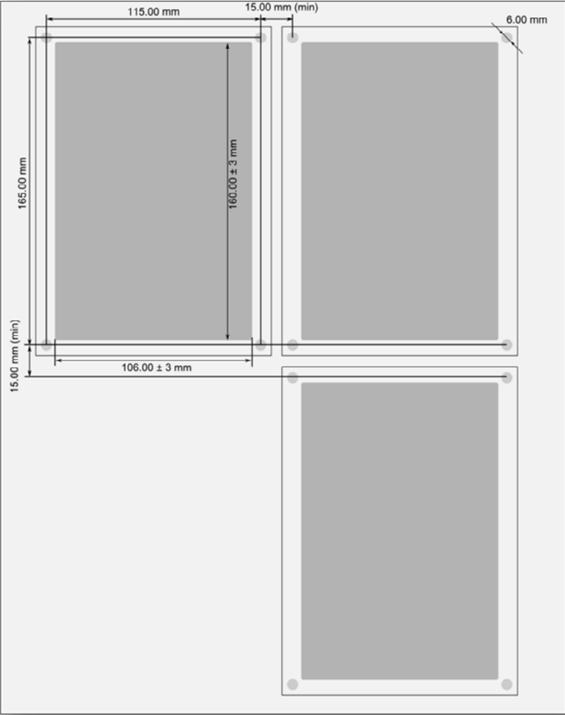
Panel cut-out and spacing of the AQ 210 series device.
