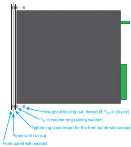
Installation of the AQ-21x device.
