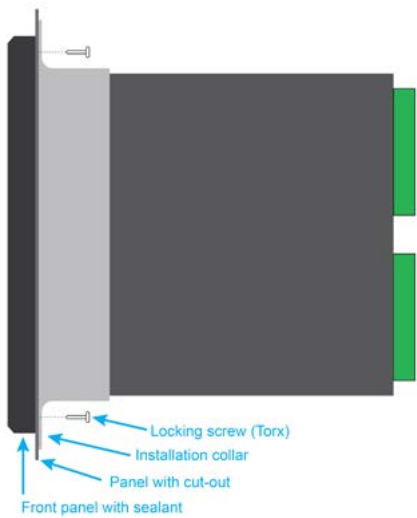
Installation of the AQ-25x device.
