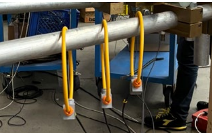
Arcteq Relays has tested Rogowski sensors in a laboratory environment for verifying performance in arc flash protection application.
