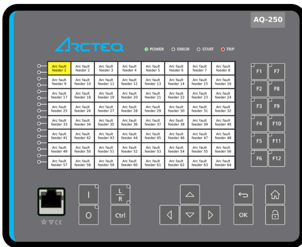
Figure. 8.8 - 43. In AQ-S254 it is possible to set up the display to show sensor activations in alarm display.
