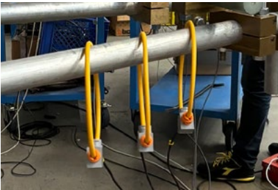
Arcteq Relays has tested Rogowski sensors in a laboratory environment for verifying performance in arc flash protection application.
