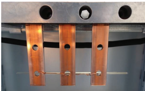
FIGURE 13. The arc initiation wire (shorting).
