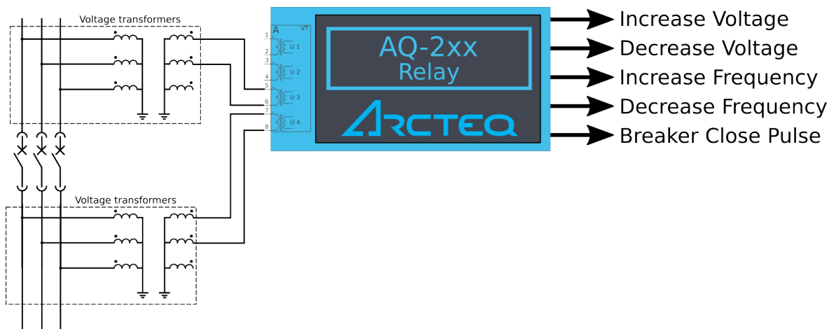
Figure. 4.5.7 - 180. Simplified presentation of synchronizer operation
