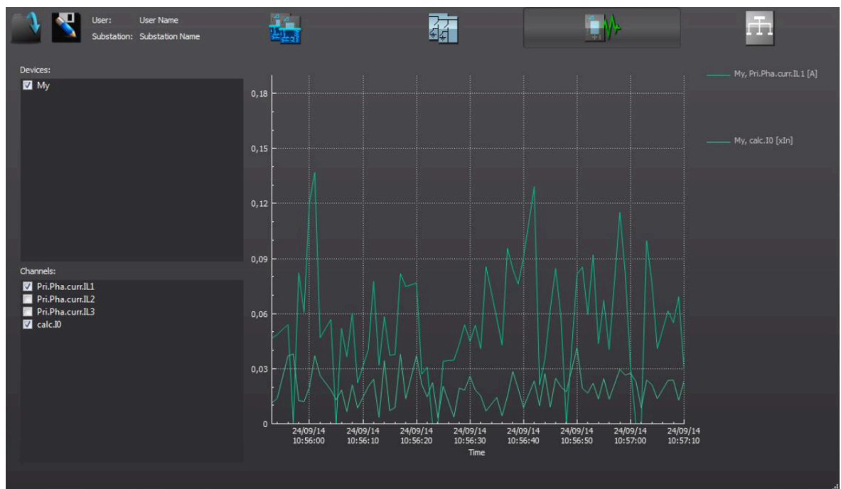
Figure. 4.6.3 - 90. Measurement recorder values viewed with AQtivate PRO.
