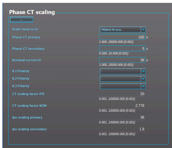
Figure. 4.2.1 - 60. Setting the phase current transformer scalings to the protected object's nominal current.
