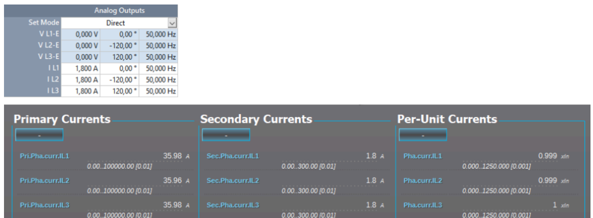
Figure. 4.2.1 - 9. Scalings display (based on the protected object's nominal current).
