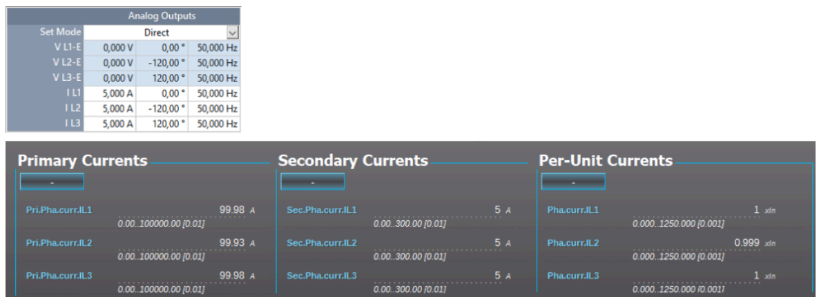
Figure. 4.2.1 - 8. Scalings display (based on the CT nominal).
