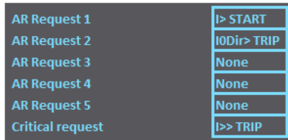
Figure. 4.5.7 - 186. Example of assigning request signals.
