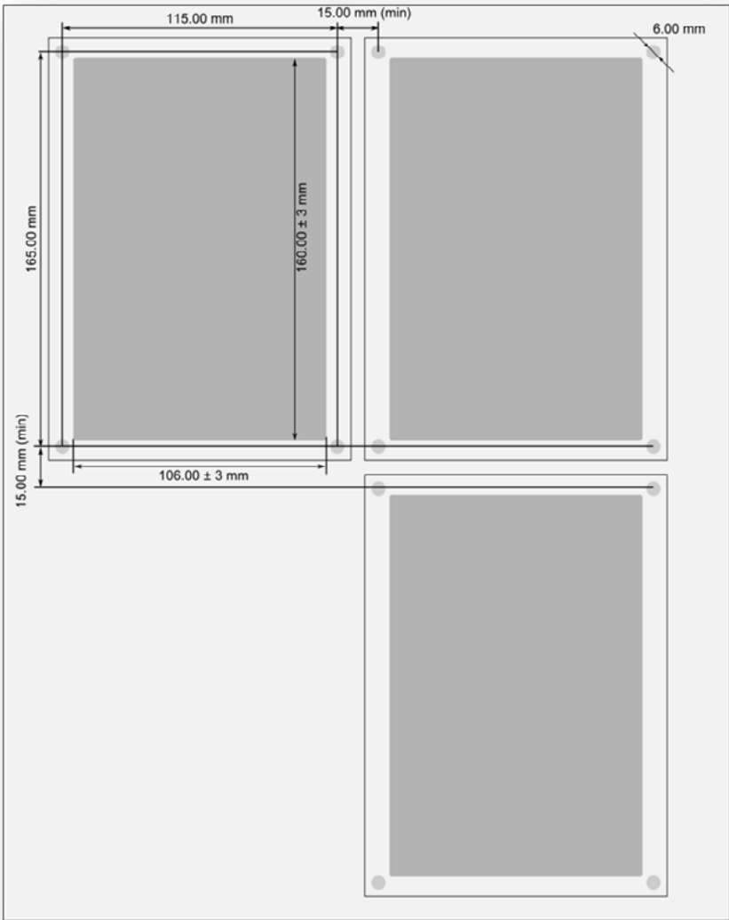
Panel cut-out and spacing of the AQ 210 seriesx device.
