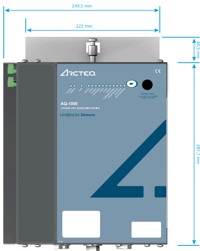
Figure. 12.2 - 40. Dimensions of AQ-1000 (when viewing the device from the front).
