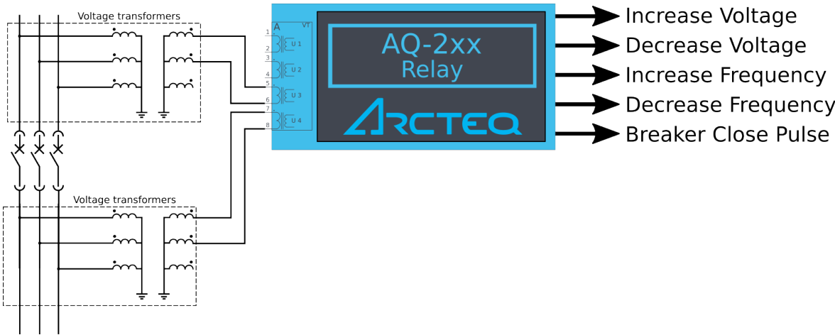
Figure. 4.5.7 - 77. Simplified presentation of synchronizer operation
