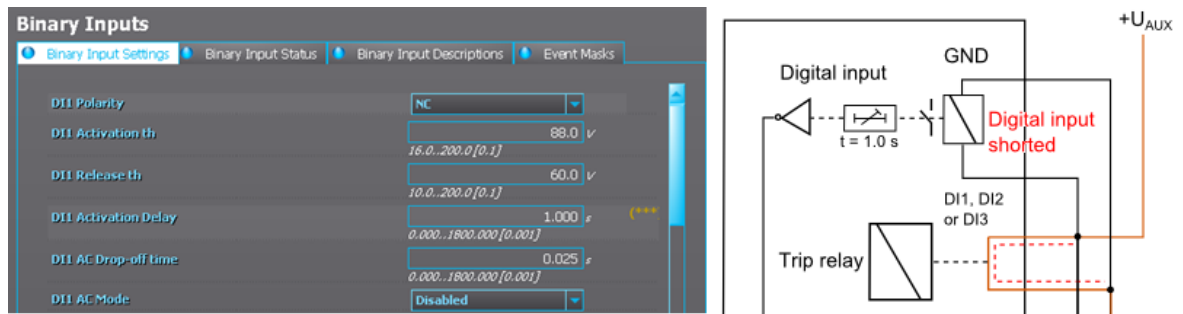
Figure. 6.3 - 210. Settings for a digital input used for trip circuit supervision.
