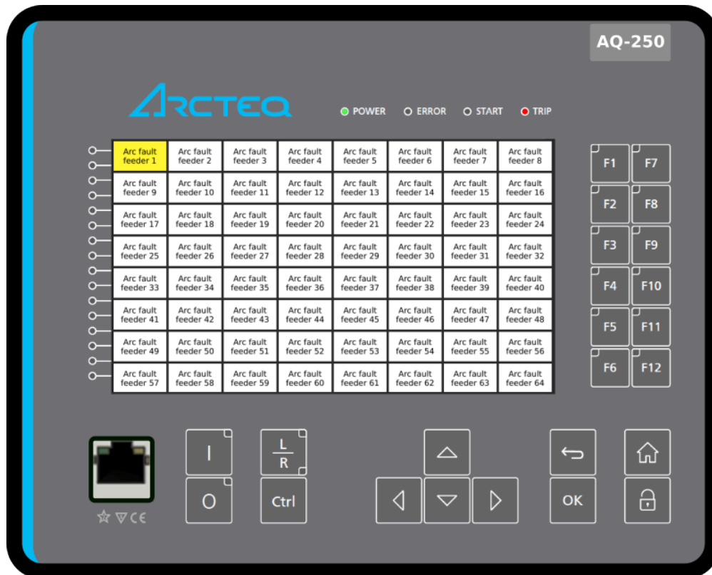
Figure. 5.5 - 27. In AQ-S254 it is possible to set up the display to show sensor activations in alarm display.
