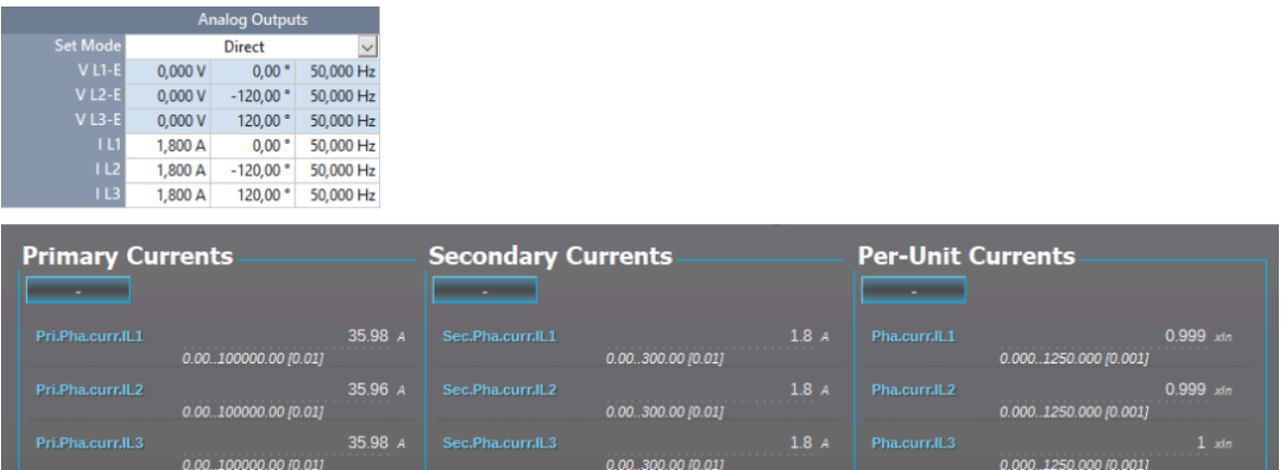
Figure. 4.2.1 - 55. Scalings display (based on the protected object's nominal current).
