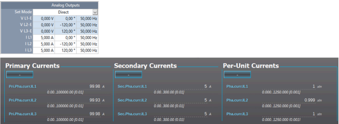
Figure. 4.2.1 - 63. Scalings display (based on the CT nominal).
