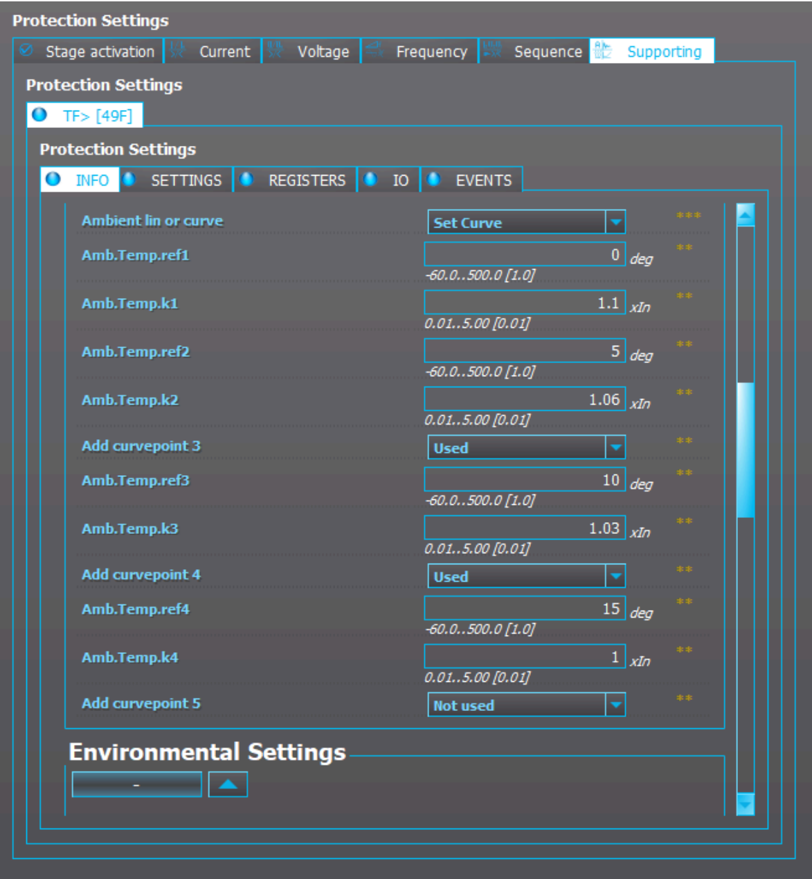
Figure. 4.4.21 - 168. Settings of the function's ambient temperature coefficient curve.
