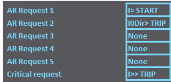
Figure. 4.5.5 - 191. Example of assigning request signals.
