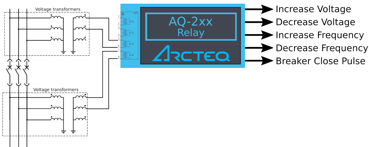
Figure. 4.5.14 - 206. Simplified presentation of synchronizer operation
