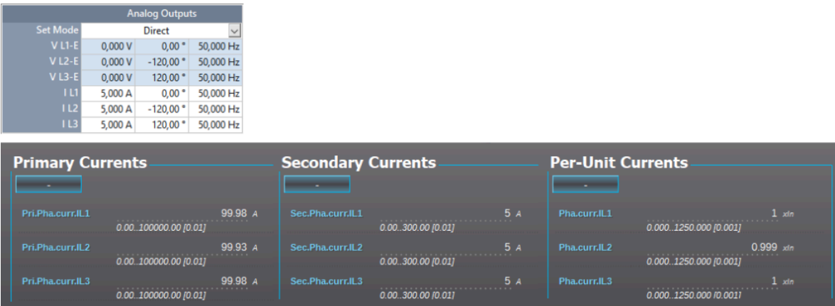
Figure. 4.2.1 - 59. Scalings display (based on the CT nominal).
