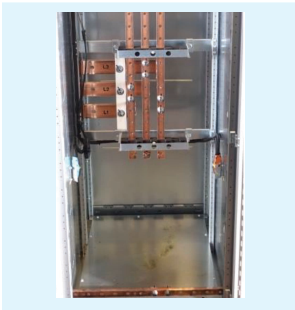
FIGURE 12. The cabinet after the 63 kA test after AQD engaged.
