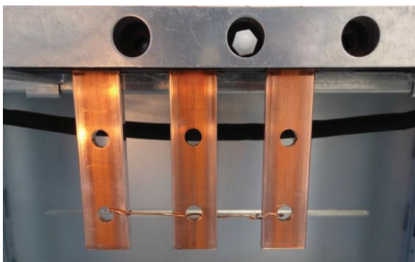
FIGURE 13. The arc initiation wire (shorting).
