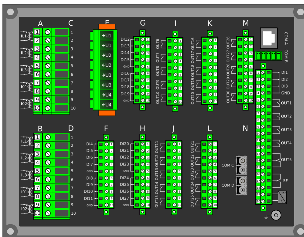
Figure. 7.1 - 215. Modular construction of AQ-X257-XXXXXXX-BBBCCCCCJ
