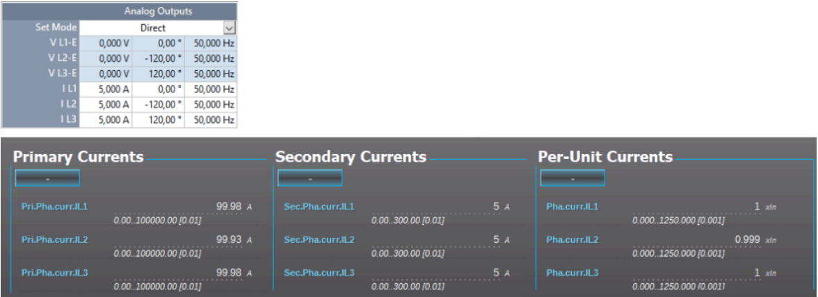
Figure. 4.2.1 - 61. Scalings display (based on the CT nominal).
