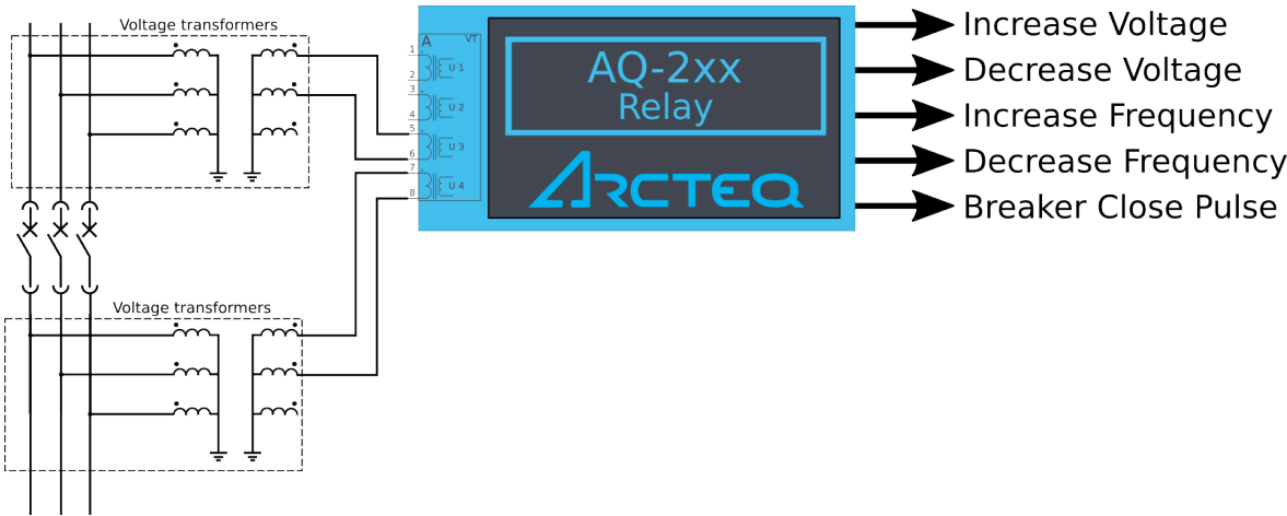
Figure. 4.5.7 - 177. Simplified presentation of synchronizer operation
