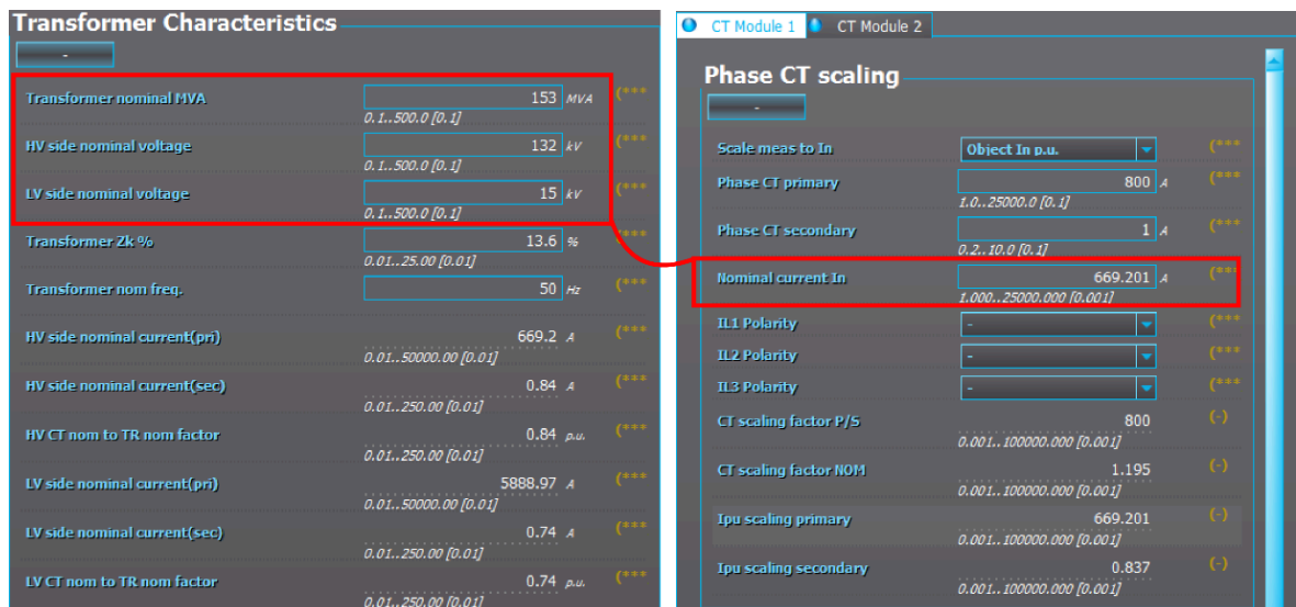
Figure. 4.2.1 - 5. Phase CT scaling to machine nominal.
