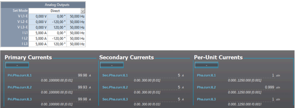
Figure. 4.2.1 - 59. Scalings display (based on the CT nominal).
