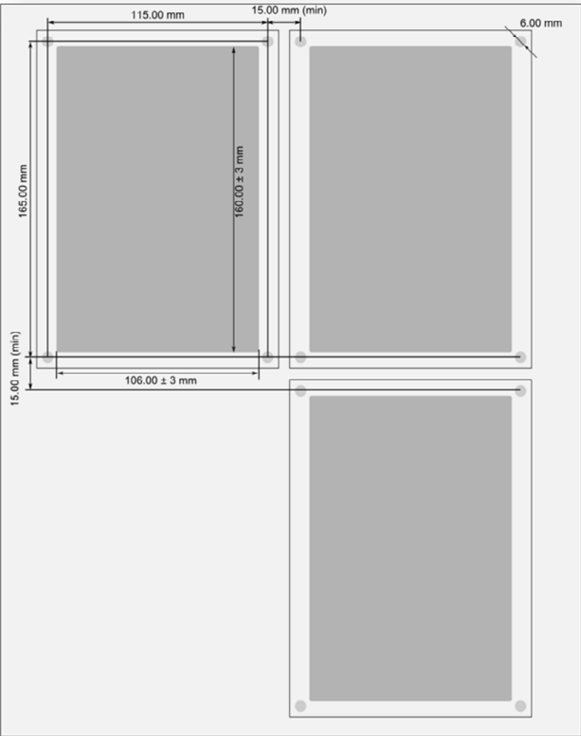
Panel cut-out and spacing of the AQ-21xx device.
