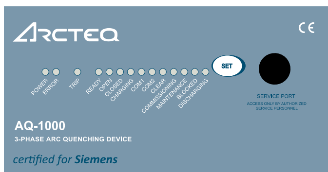
Figure. 6.2.1 - 17. The front panel of AQ-1000 (top half).
