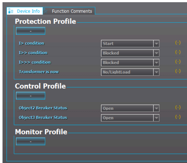
Figure. 6.2 - 38. Checking the function states in the General menu while in Live Edit mode.
