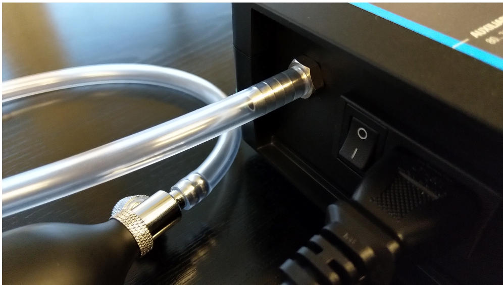
Figure. 5.1 - 9. Connecting the hose of the pressure pump to the control unit.
