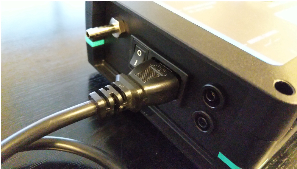
Figure. 5.1 - 10. Connecting the auxiliary power cable to the control unit.
