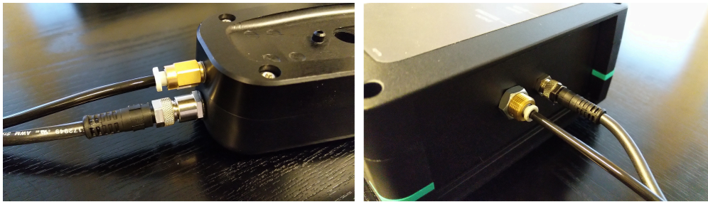
Figure. 5.1 - 8. Connecting the injector to the control unit.
