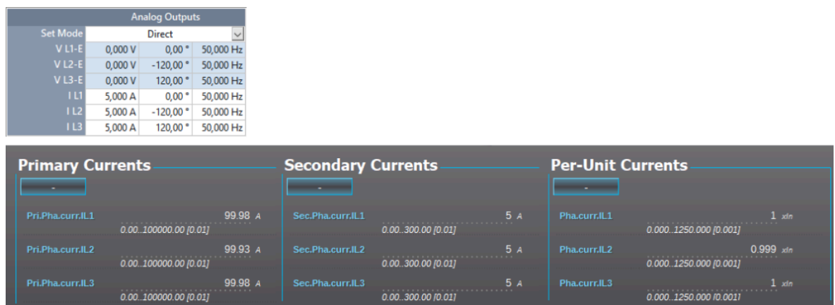
Figure. 4.2.1 - 61. Scalings display (based on the CT nominal).
