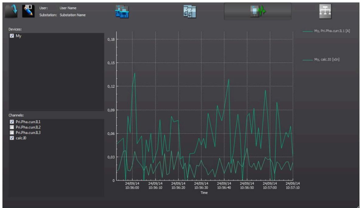
Figure. 4.6.7 - 236. Measurement recorder values viewed with AQtivate PRO.
