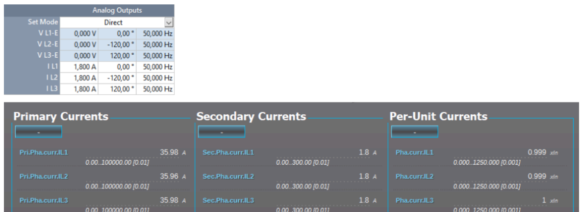
Figure. 4.2.1 - 62. Scalings display (based on the protected object's nominal current).
