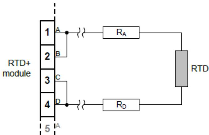
Figure. 10.9 - 61. 3-wire RTD wiring.
