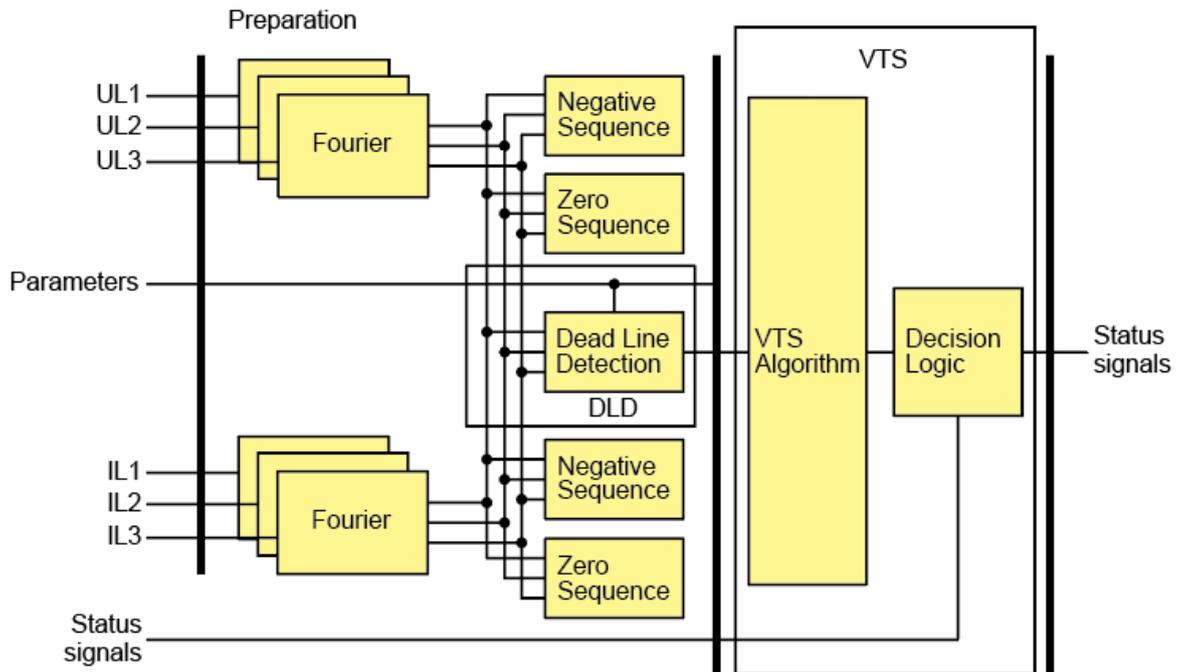
The voltage transformer supervision logic operates through decision logic presented in the following figure.
