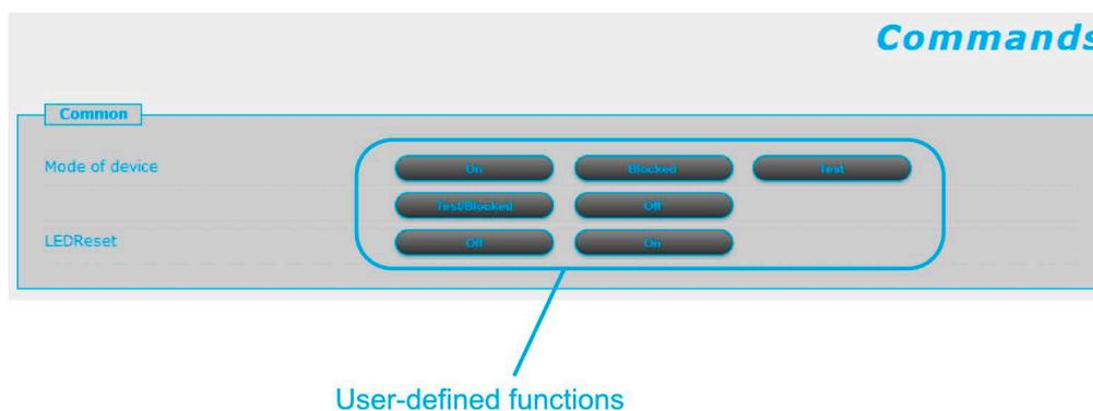
In the commands menu you can instruct the processor to carry out customized, user-defined commands. You can use the various mode buttons (**On**, **Blocked**, **Test**, **Test/Blocked**, **Off**) and LED buttons (**On**, **Off**) to define functions. A status update is always generated with a command, regardless of whether the command was successful or not. If the command was unsuccessful, the device gives the reason for the error.
