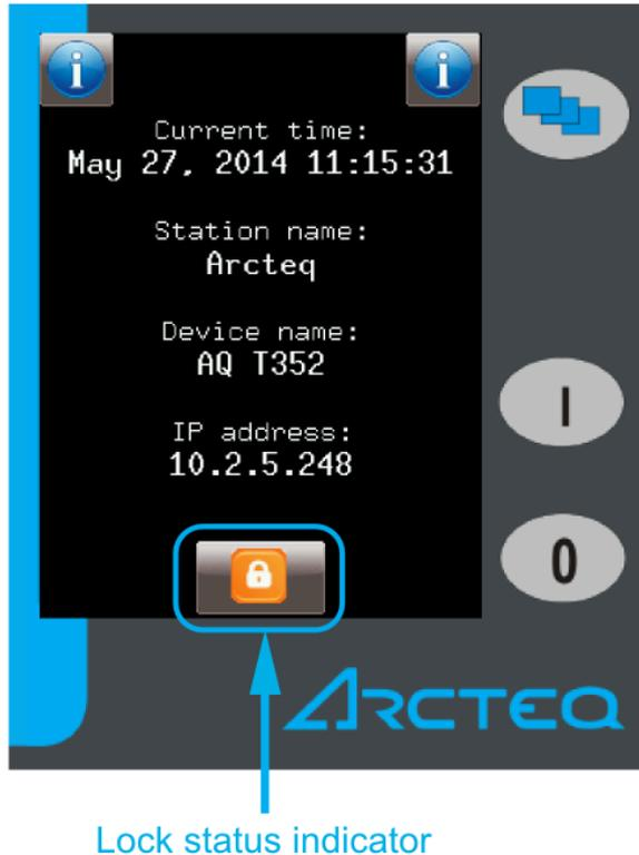
The **lock status indicator** shows whether a password is required to unlock the device before parameters or settings can be changed. By default, the device is not password-protected. However, if such a functionality is needed, you can set the password application via the web interface.
