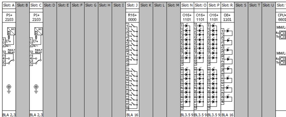
Example above presents a simple hardware configuration with redundant power supplies (PS+2103), signaling binary outputs (R16+0000), binary input cards (O16+1101 and O8+1101) and 100Base-FX Ethernet MM/LC communication card (CPU+6601).
