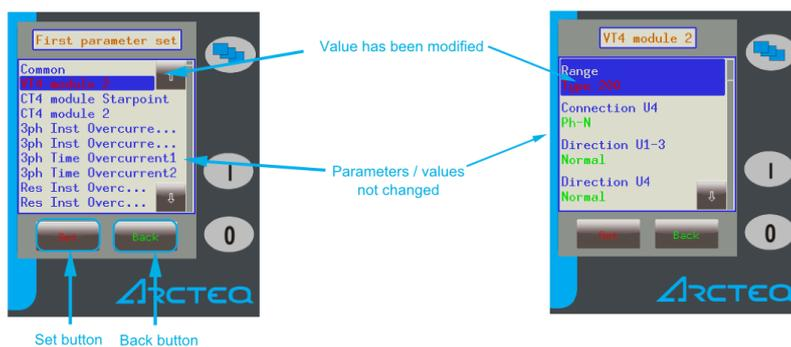
Normally, the various function blocks appear blue. However, if any value has been changed within a function block, its listing appears red to notify the user. This also happens in the function block screen, where unmodified parameter values appear green but modified values appear red.
