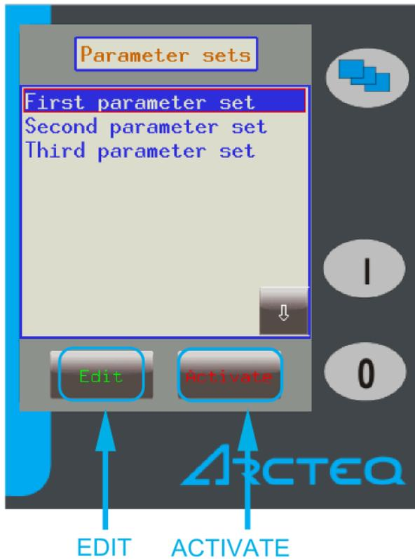
The **Activate** button activated the selected parameter set, which the device will now use. Depending on the device's configuration, the "Activate" button may not be available. The **Edit** button takes you to another screen where you can choose which function blocks the parameter set uses. Please note that when there is only one parameter set, the device takes you immediately to the parameter set edit screen (below).
