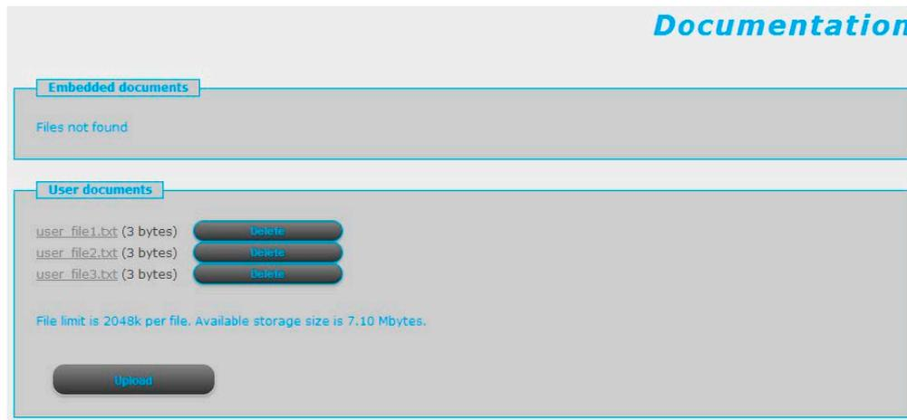
This page displays the documentation files on the device. You can upload other documents and files on the device, which are then saved and can be accessed later. One file can be up to 2048K , and there is storage for up to 8 MB of documentation.
