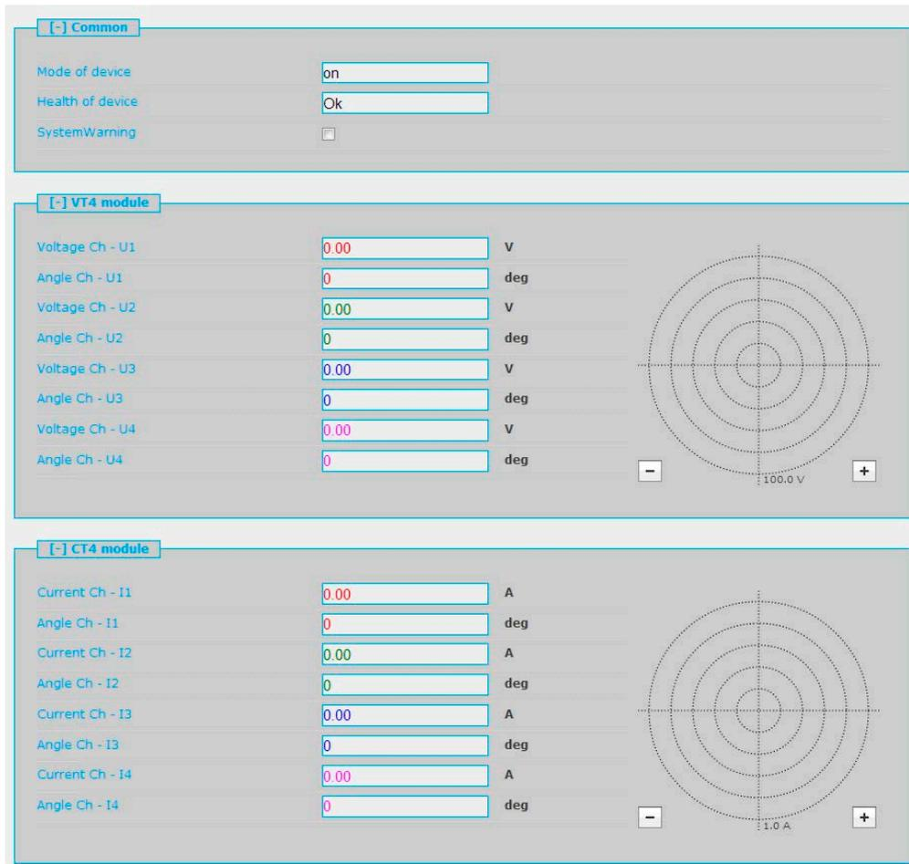
This menu displays the data measured by the device. Each block has their own section, and these sections can be expanded and collapsed individually as needed with the [+] and [-] signs in front of their names. The values on screen are updated every second, which may cause older systems to slow down or halt the browser altogether. All data is strictly read-only, and cannot be modified. If there is a counter on the page, next to it will be a button that resets it.
