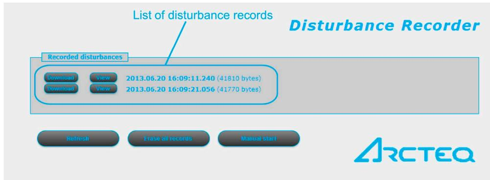
The "Recorded disturbances" section lists all disturbance records. You can refresh the list with the **Refresh** button to display any new disturbance records that have occurred after the page was opened or refreshed last. You can also clear the list with the **Erase all records** button. Additionally, you can create a disturbance record manually by clicking the **Manual start** button.
