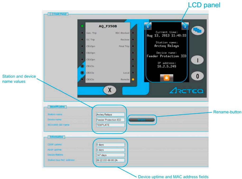
In the main menu you can control the device's front panel. The image of a touch screen (located on the right) behaves the same way as the actual touch screen. For more information on the touch screen, please refer to the "Touch screen" subchapter in the "IED user interface" main chapter.
