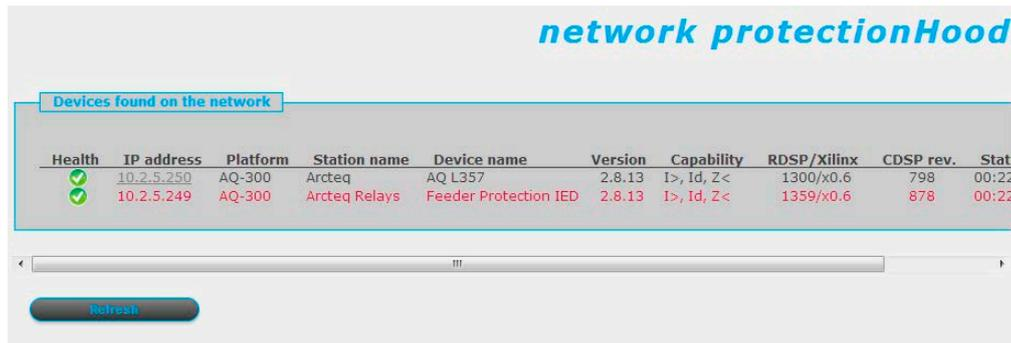
This page shows all other devices that are located in the same network with the AQ-300 unit. The page identifies compatible devices and displays information about them, such as their IP address and version. The device that is currently accessed is highlighted in red in the list. You are redirected to other devices by clicking their corresponding links. The **Refresh** button scans the network for connected devices.
