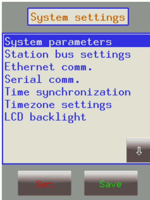
In the system settings menu you can set certain parameter values that are related to the device itself (as opposed to its protection functions and operations). The menu works similarly to the parameters menu and the same properties apply.
