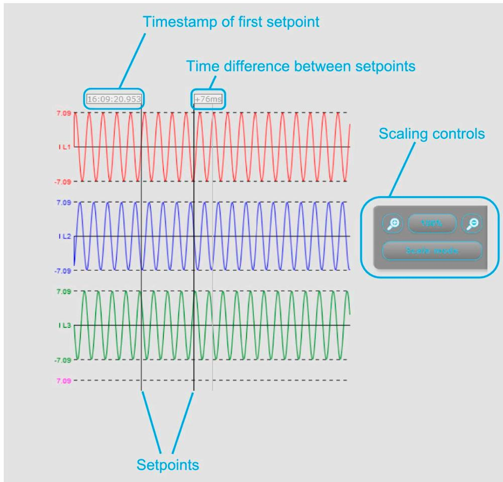
You can set a setpoint by clicking anywhere on the graph, and the positioning the cursor to a desired second point. The preview then displays the timestamp of the first setpoint, and the time difference between the two setpoints. You can also scale the time axis with the scaling controls (the plus and minus magnifying glasses), or by clicking the **Scale mode** button to switch between standard and scaled modes. The scaled mode stretches the Y axis of all recorded values.
