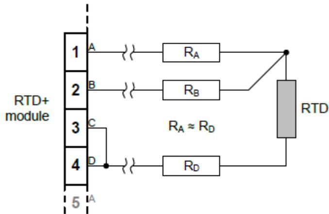
Figure. 10.9 - 62. 4-wire RTD wiring.
