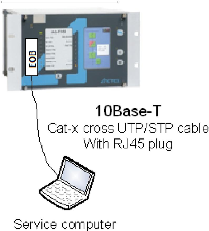
Please note that the RJ45 connector can also be connected to an Ethernet switch. When this is the case, all the network's IEDs with client functionalities (e.g. a computer) have access to the device.
