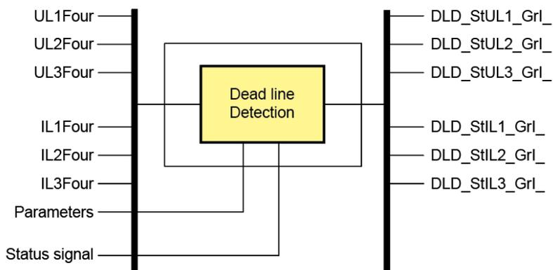
The function block of the dead line detection function is shown in figure bellow. This block shows all binary input and output status signals that are applicable in the AQtivate 300 software.
