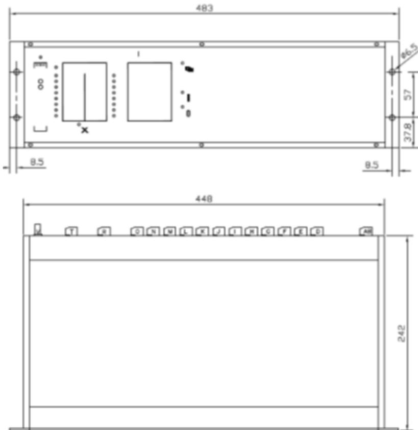
Figure. 10.12 - 67. Panel cut-out and spacing of AQ-x39x IED.
