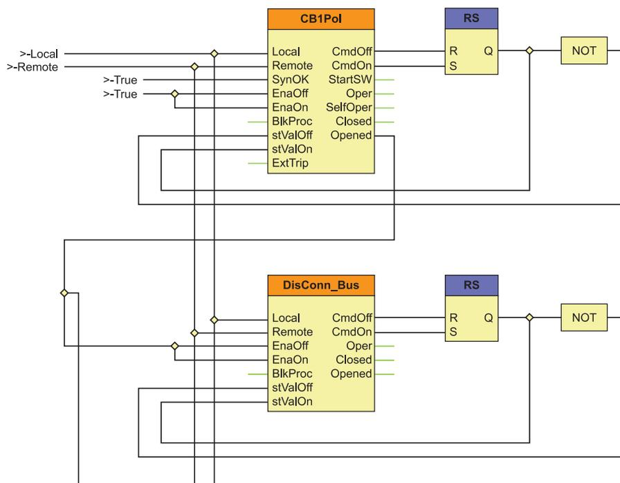
In the Figure above the local/remote selection is made by another function block (Common). The disconnector cannot be switched any time: interlocking is needed; the “EnaOff” and “EnaOn” are programmed for the “Opened” state of the circuit breaker. The function block does not need to be blocked; the “BlkProc” input is not connected. The disconnector is simulated by an RS flip-flop, the status inputs are connected to the simulated signals.
