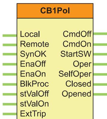
The binary input and output status signals of the circuit breaker control are listed in tables below.
