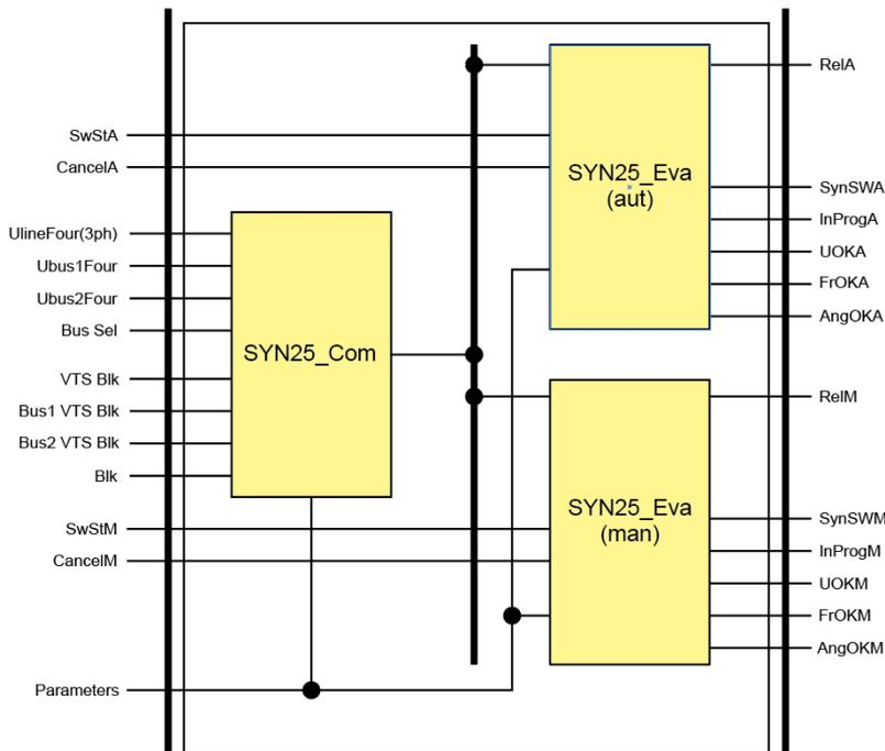
The synchro check/synchro switch function contains two kinds of software blocks:
