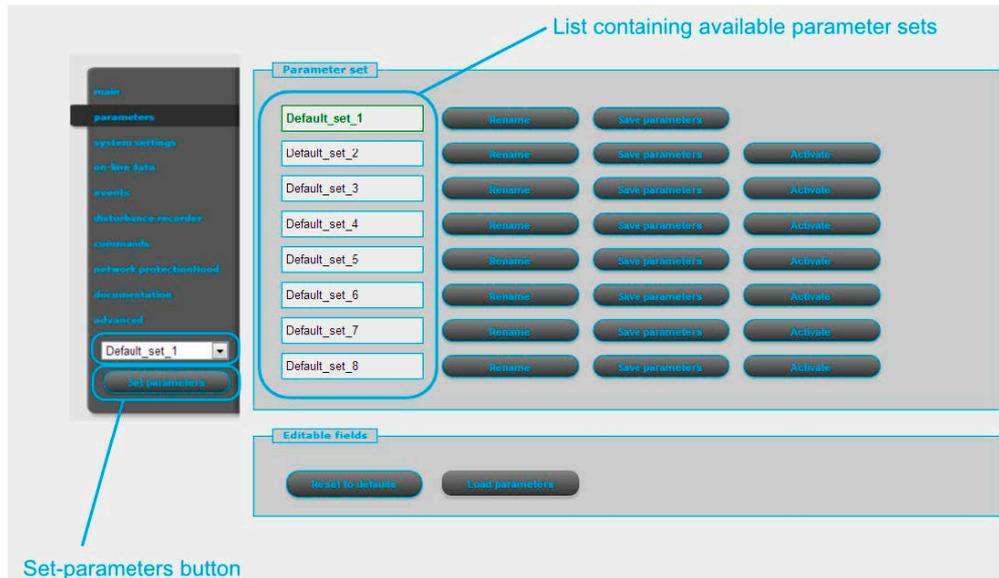
With the **Activate** button, you can enable the selected parameter set. The device will now use the values from this set. The **Rename** button, unsurprisingly, renames the selected parameter set. The names can include alphanumeric characters, spaces, dashes and underscores. Please note that two or more parameter sets **CANNOT** share the same name! The **Save parameters** button saves the selected parameter set in a separate file, which can be loaded into the device at any time.
