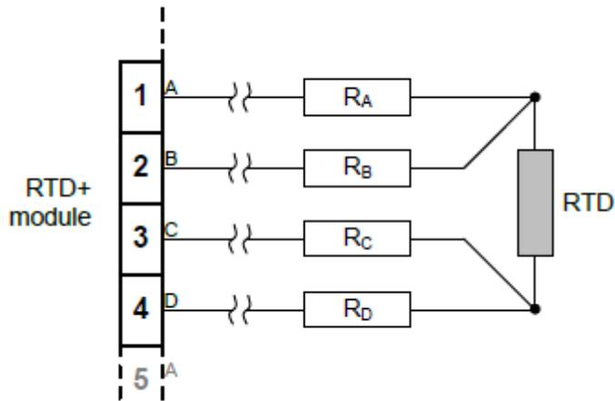
Figure. 10.9 - 63. 4-wire RTD wiring. of potentiometer.
