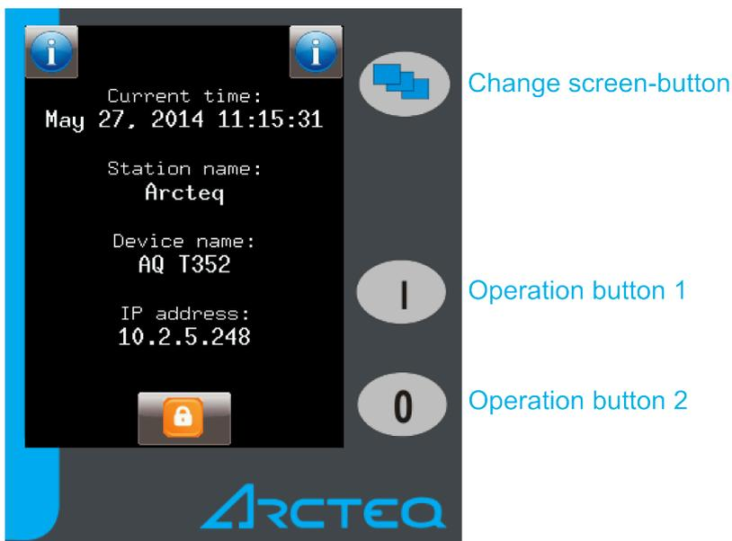
The touch screen is the main control where you can enable functions and input values.
