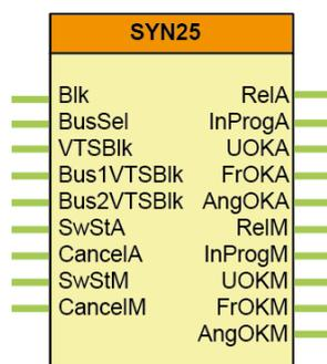
The progress is indicated by the output status signal (SynInProgr Auto/Manual). The started command can be canceled using the input signal (Cancel Auto/Manual).
