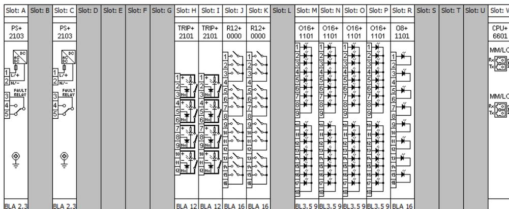
Example above presents a simple hardware configuration with redundant power supplies (PS+2103), trip contacts (TRIP+101), signaling binary outputs (R12+0000), binary input cards (O16+1101 and O8+1101) and 100Base-FX Ethernet MM/LC communication card (CPU+6601).
