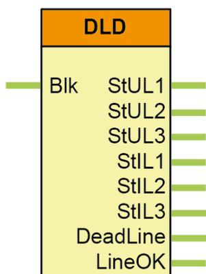
The binary input and output status signals of the dead line detection function are listed in tables below.
