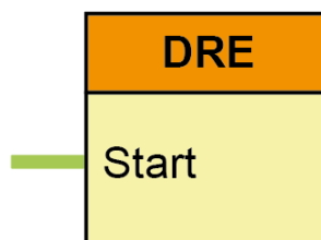
Figure. 6.4.11 - 126. The function block of the disturbance recorder function.
