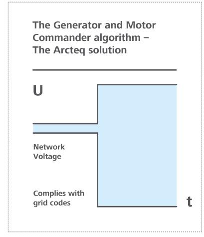
Common solution in the market where MVar control will follow the network voltage dip. The Commander compensates the network dip by applying AVR and MVar control modes simultaneously.
