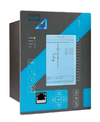
The AQ-F215 feeder terminal is equipped with the intermittent earth fault protection. The protection algorithm combined with 0.2S measurement class and 3,2 kHz sampling frequency, enables it to detect and isolate intermittent earthfaults with high accuracy.
