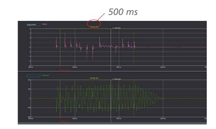
The triptime of the intermitten earth fault protection is set to 500 ms. Fom this disturbance record from AQ-F215 relay can be read that the relay detects the intermittent earth faults and trips within the set time.
