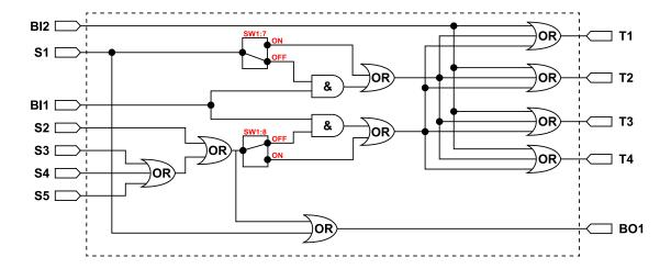
Figure. 4.4.2 - 10. The DIP switch settings for SS:0.
