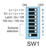
Figure. 4.4.2 - 14. The trip logic matrix for SS:1.
