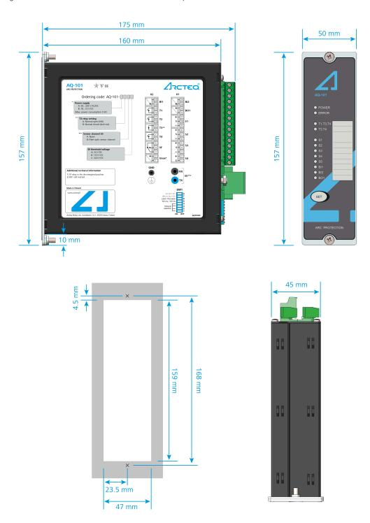
Figure. 3.2 - 3. Dimensions of the DIN rail variant of the device.
