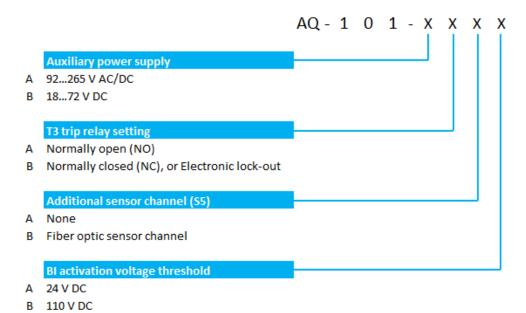
AQ-101D point sensor unit (DIN rail mounted)
