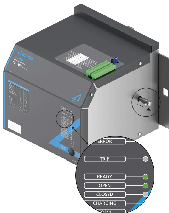
Figure. 6.2.2 - 16. Operating mode "Ready".
