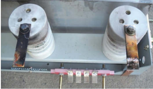
Figure 13 - There is limited damage to the pT drawer after an arc flash. (photo courtesy of Shallbetter, Inc.)
