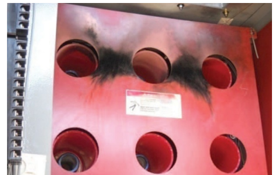
Figure 11 - The breaker test damage results show only carbon residue. (photo courtesy of Shallbetter, Inc.)
