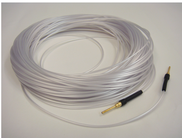
Figure. 5.4. - 13. AQ-07 sensor with covered ends.
