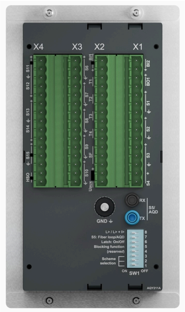
Figure. 8. - 17. Connections of the AQ-103(LV) basic variant (with SF in de-energized position).
