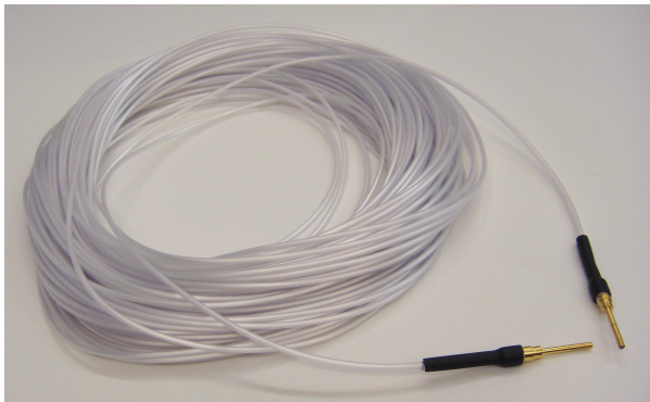
Figure. 5.5. - 14. AQ-08 sensor with covered ends and terminals.
