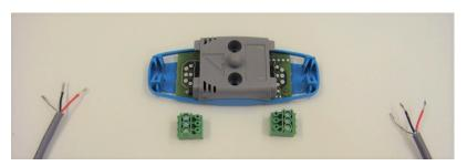
2. Before connecting the cable to the connector, make sure that the connecting order is correct (+, signal, shield). You can check the appropriate pins from the sensor, as the information is shown on the inside of the sensor's blue plastic cover (see the circled are in the image below, on the left). Next, plug the wires into the connector and fasten them with a screw driver (see the image below, on the right). Repeat for the other connector.
