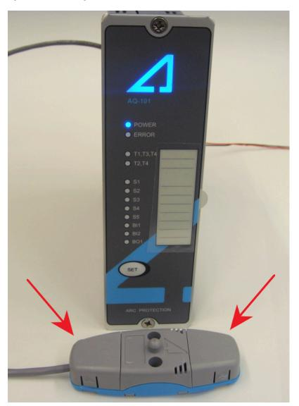
You can connect a maximum of three (3) point sensor in a series on one sensor channel (see the image below).
