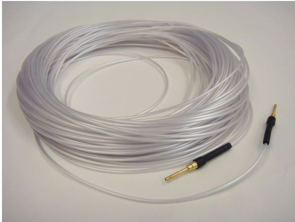
Figure. 5.2. - 8. AQ-07 sensor with covered ends.
