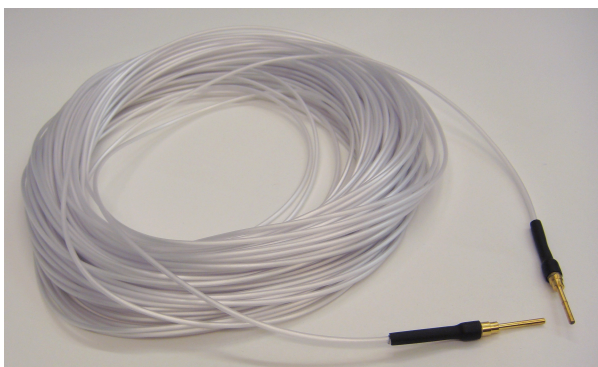
Figure. 5.3. - 9. AQ-08 sensor with covered ends and terminals.
