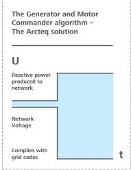
Traditional solutions where MVAR control will follow the network voltage dip. The Commander compensates the network dip by applying AVR and MVAR control modes simultaneously.
