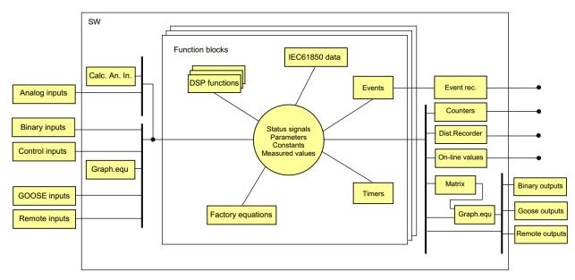
Figure 1-7 The HW and SW structure of the AQ-300 devices.
