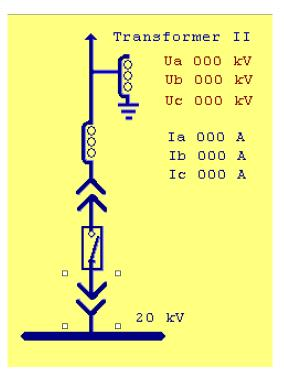
Figure 3-2 Required user screen for a transformer bay
